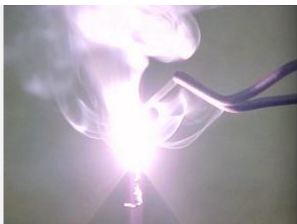
Magnesium metal 'turns into' a white powder: Magnesium Oxide
